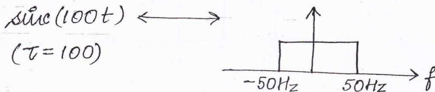
— Nyquist freq. =  $2 \times 50\text{Hz} = 100\text{Hz}$
